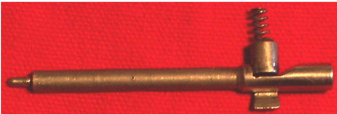
Figure 6-2. Proper Orientation of Firing Pin Parts
