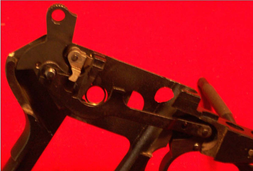
Figure 7-8. Trigger Bar / Disconnecter Orientation with Sear
