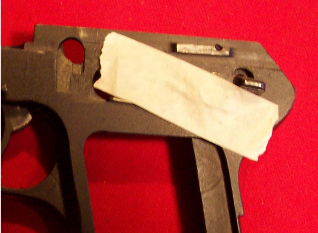
Figure 7-4. Safety Positioning for Sear Installation
