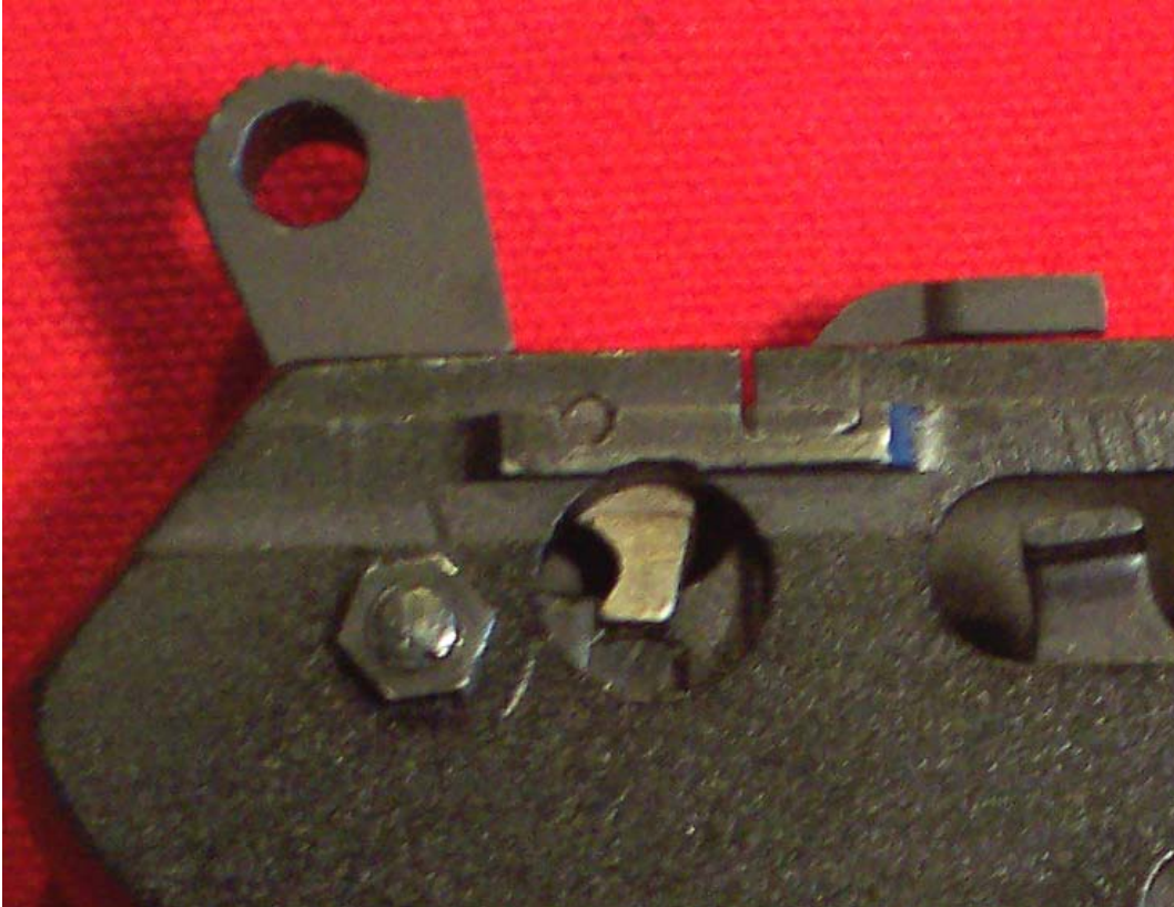
Figure 7-11. Proper Trigger Bar/Disconnecter and Sear Engagement.
