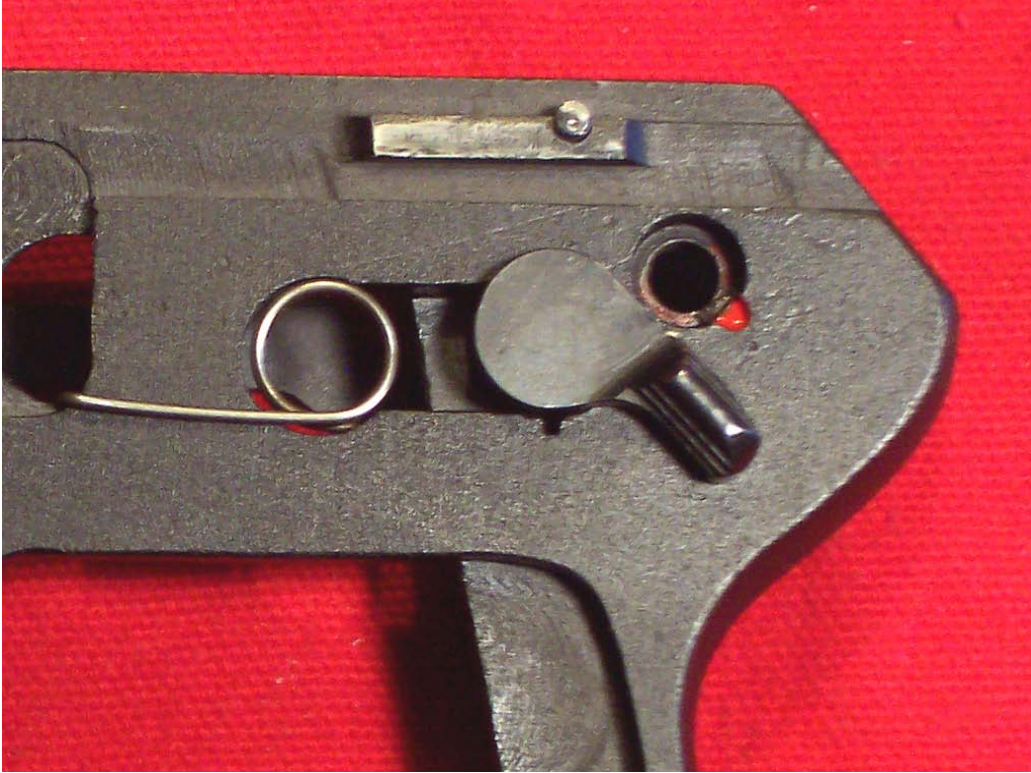
Figure 7-6. Safety Position for Hammer Installation
