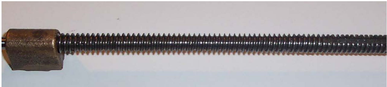
Figure 1. Lead Screw Removed from Lathe Shows Severe Wear with Pointed Threads
